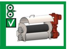
Gripping and non-gripping rotation direction when both protection covers are closed
